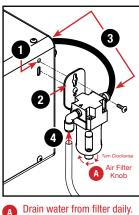
Drain water from filter daily. Turn knob clockwise (from top view) to open. Drain. Turn knob counter-clockwise to close valve. 1. Remove top screw from hole.
