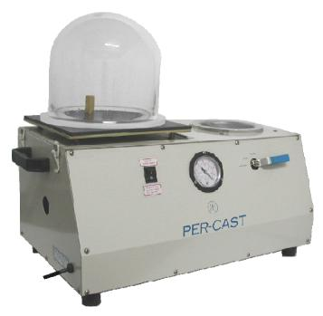
**Feature**: This vacuum investment machine can also be used as a vacuum casting machine.
