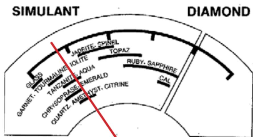
When the indicator stops at the above position, the stone tested may be Quartz, Amethyst, Citrine, Tanzanite or Aqua, i.e., any stones that fall within the white strip that the indicator passes.
