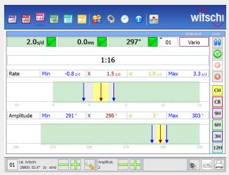
The Vario mode measures the rate and amplitude stability over a longer time range. Each numerical measurement is represented by an arrow on the linear scale.
