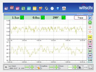
In this mode, the rate deviation and the amplitude are recorded in parallel in graphical format. The Trace mode provides long-term measurements up to 100 hours. This provides an extended time range (e.g. power reserve cycle) for measuring movements.
