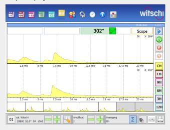
The Scope function graphically displays the acoustic beat noise of the watch. A detailed analysis of the beat noise, i.e. of the state of the escapement, can be carried out. The display can be switched from one to two horizontal axes. Thereby, the averaging of the signals of 1, 10, 20 and 50 beat noises is possible.
