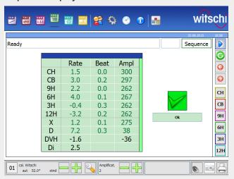
This neatly structured table clearly displays the measurement results in each position as well as the average and the largest difference between all positions and particular ones.
