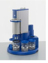
The Elmasolvex<sup>®</sup> SE cleaning machine is a manual cleaning machine for cleaning watch movements and other mechanical precision parts witch aqueous solution and solvent based cleaning and rinsing media.
