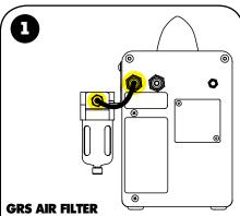
Connect the air filter to the GraverSmith by loosening the side cover screw and sliding the bracket onto the screw. Re-tighten screw.
