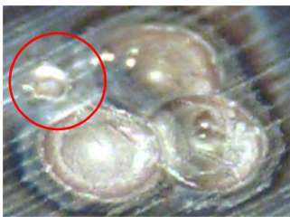
Electrode contamination can lead to small "explosions" that create craters in the workpiece. All four welds were made at the same setting. Metal contamination on the electrode caused one weld to create a crater.
