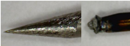
Electrode contamination can lead to small "explosions" that create craters in the workpiece. All four welds were made at the same setting. Metal contamination on the electrode caused one weld to create a crater.
