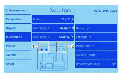
Fig. 36: Assigning functions
