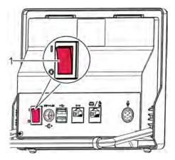
Fig. 14: Switching off the Watch Expert
