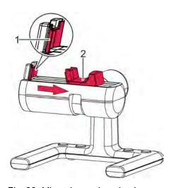
Fig. 22: Microphone clamping jaw
