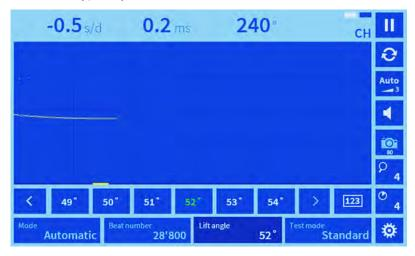
Fig. 17: Selecting a lift angle manually
