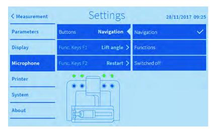
Fig. 35: Setting up navigation buttons
