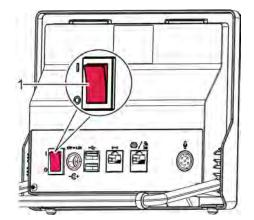
Fig. 13: Switching on the Watch Expert
