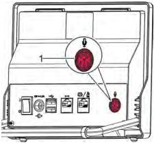
Fig. 42: Removing the microphone cable
