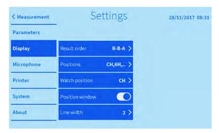
Fig. 33: Hiding/displaying the position windows of the measured test positions in the main display (only in the diagram display mode)
