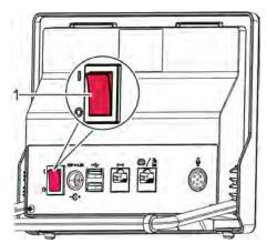
**1.** Set the switch (Fig. 41/1) to the *[O]* position.
