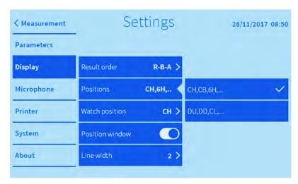
Fig. 31: Setting test position designation types
