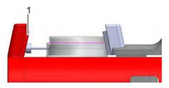
Fig. 24: Clockwork clamped in cup
