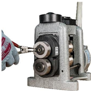
Remove black circlip (ring)
