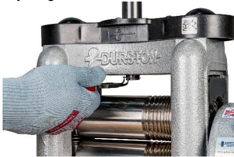
Remove black circlip (ring) on shaft
