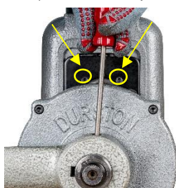
Undo screw in turning handle and slide off
