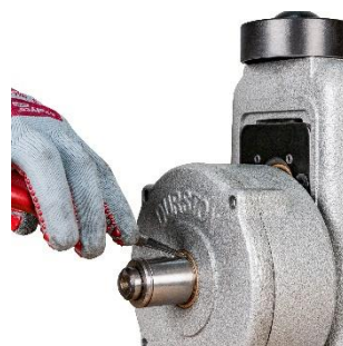
Remove 4 screws and remove circlip (ring)
