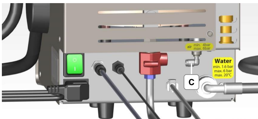
Figure 4.3.2: Connection for compressed air (without blind plug)
