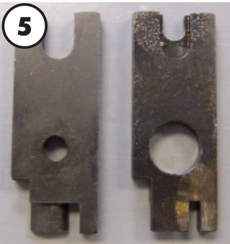
1. Using a 3/16" allen head wrench, remove the bolt holding the movable cutter bar # 004-295
