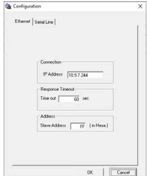
Figure 39.1. The Modbus Configuration screen.
