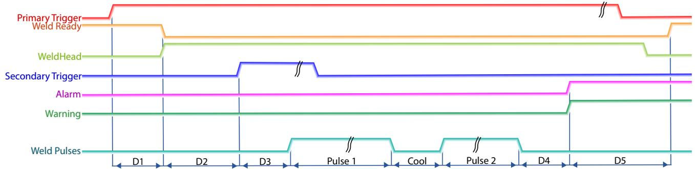
Figure 21.1. Sample timing diagram for Fully Manual scenario.
