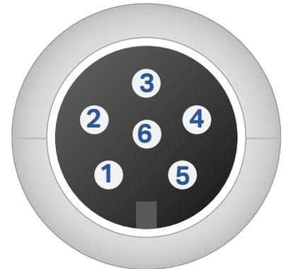
Figure 57.1.E-STOP pin-out.
