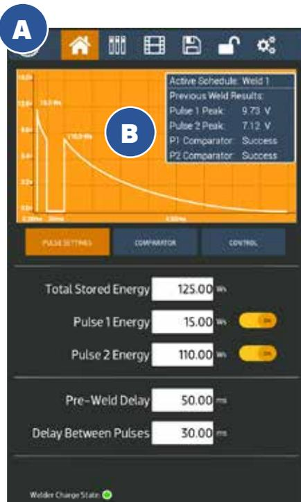
Figure 13.1. Homescreen with Pulse Settings Tab selected. See Chapter 4 for specific details about the Home Screen.
