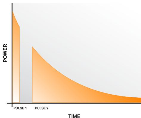
Figure 16.2. Example of dual pulse energy discharge curve.
