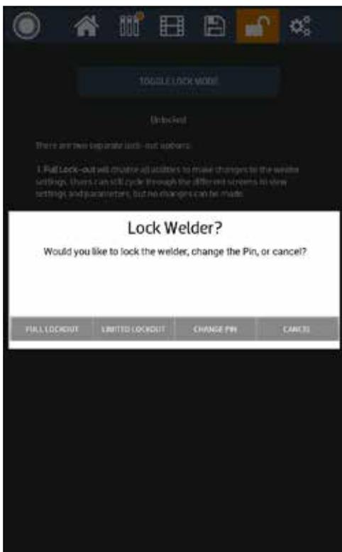
Figure 32.1. You can lock the CDDP-A, which prevents other operators from either using the welder or changing the weld settings.
