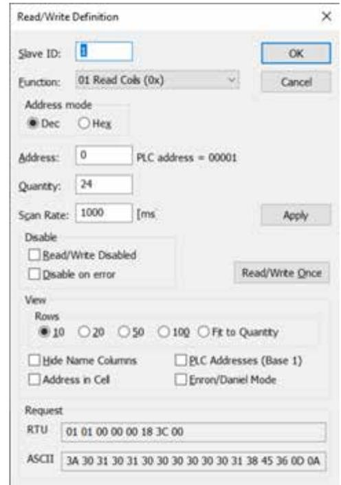
Figure 45.1. Read/Write Definition window.
