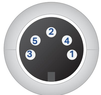
Figure 57.3.Primary Trigger pin-out.
