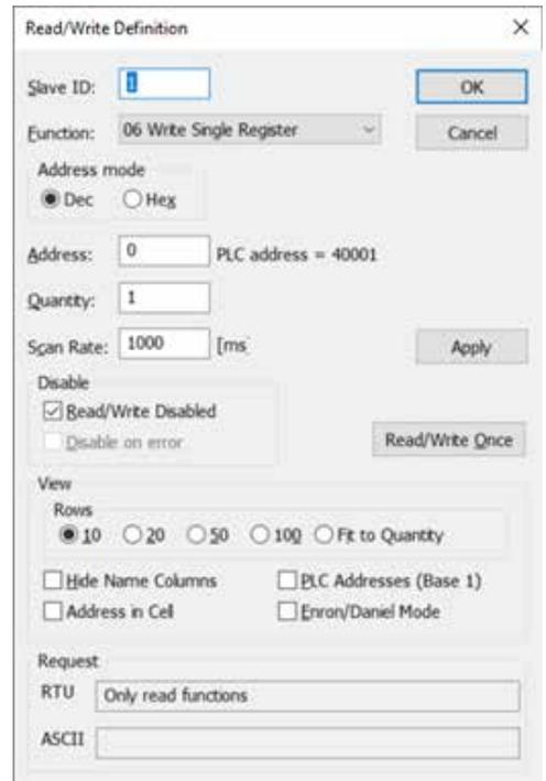
The screenshot shows the 'Read/Write Definition' dialog box. The 'Function' dropdown is set to '06 Write Single Register'. The 'Address' field contains '0', with a note 'PLC address = 40001'. The 'Quantity' field contains '1'. The 'Scan Rate' is '1000 [ms]'. Under the 'Disable' section, the 'Read/Write Disabled' checkbox is checked. The 'View' section has 'Rows' set to '10'. The 'Request' section has 'RTU' set to 'Only read functions'.
