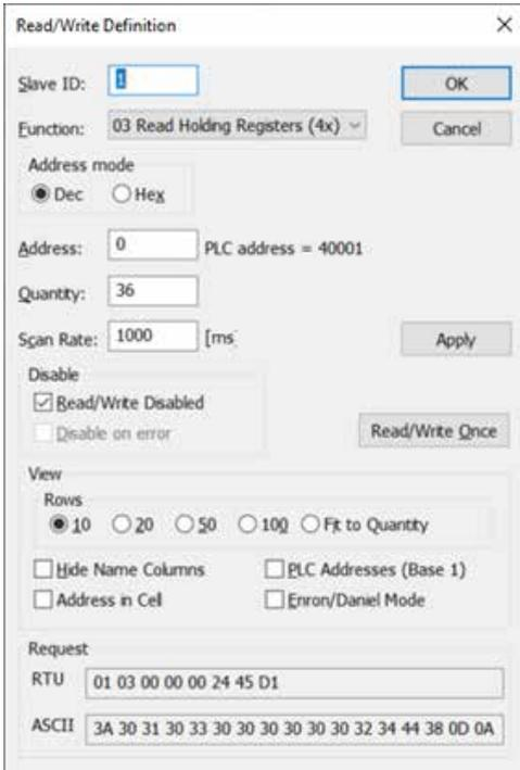
Figure 46.1. Read/Write Definition window.
