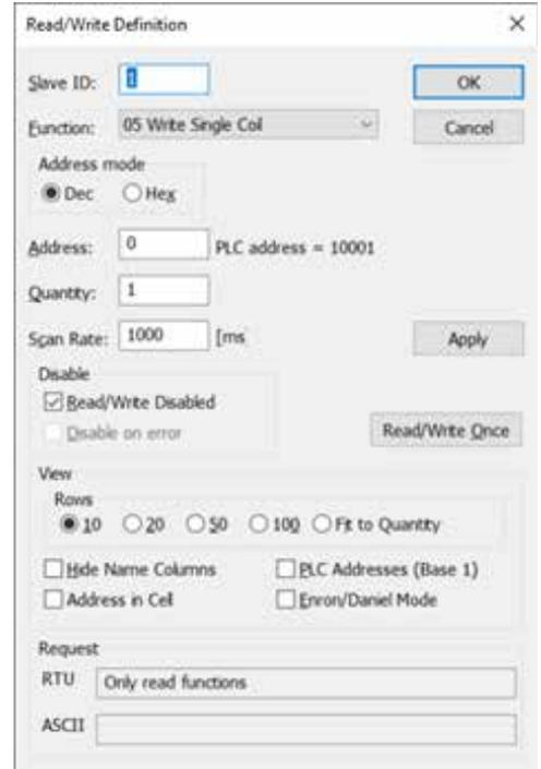
The screenshot shows the 'Read/Write Definition' dialog box. The 'Function' dropdown is set to '05 Write Single Coil'. The 'Address' field contains '0', with a note 'PLC address = 10001'. The 'Quantity' field contains '1'. The 'Scan Rate' is '1000 [ms]'. Under the 'Disable' section, the 'Read/Write Disabled' checkbox is checked. The 'View' section has 'Rows' set to '10'. The 'Request' section has 'RTU' set to 'Only read functions'.
