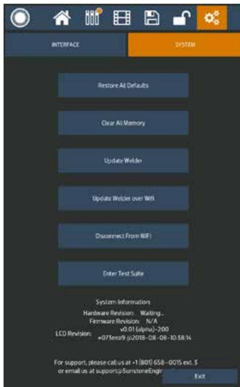
Figure 34.1. The Settings Screen can be used to make changes to the general power supply settings.
