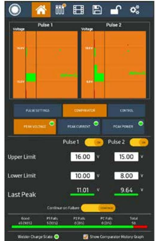
Figure 19.1. Histogram of previous welds.
