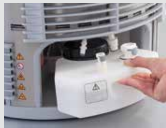
Installing media containers
