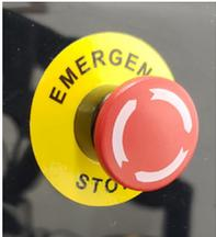
Figure 10.1. Make sure the Emergency Stop Button is disengaged.
