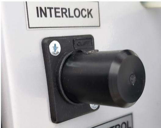
Figure 8.2 Insert the Interlock into the Interlock port found on the rear of the welder.
