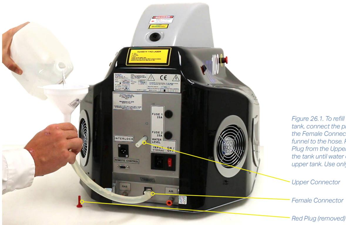
Figure 26.1. To refill the cooling tank, connect the plastic hose to the Female Connector. Connect the funnel to the hose. Remove the Red Plug from the Upper Connector. Fill the tank until water comes out of the upper tank. Use only deionized water.
