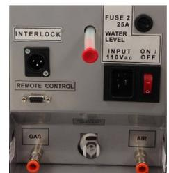
Figure 9.4. The final step to filling the tank is replacing the Red Plug on the end of the Upper Connector.
