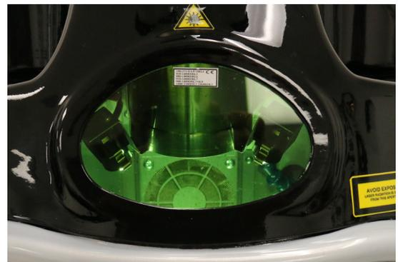
Figure 31.2. Weld Chamber Infrared Filter.
