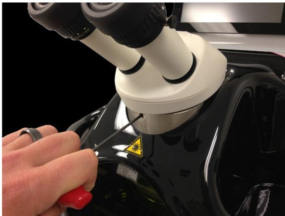
Figure 24.1. Before realigning the crosshairs, make sure the microscope is firmly attached to the welder.
