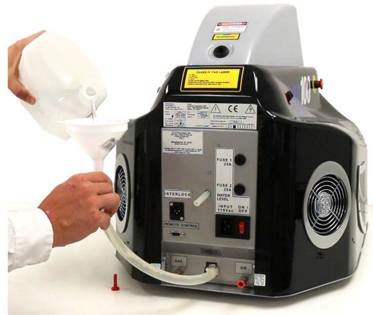
Figure 9.3. To fill the welder with coolant water, attach the funnel, tube, and connector to the bottom Female Connector “Remove Water” Port. Remove the Red Plug from the Upper Connector tube. Fill the welder with deionized water that comes with the Orion LZR laser welder.
