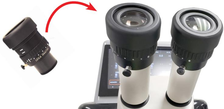
Figure 9.2 Attach eyepieces to the microscope tubes and tighten the screws with an Allen wrench. Generally speaking, the eyepiece with the crosshairs is attached to the right tube.
