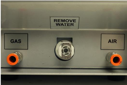
Figure 8.1 Gas Inlet Connections. Argon shield gas is connected to the "Gas" inlet on the left; compressed air may be connected to the "Air" inlet on the right.
