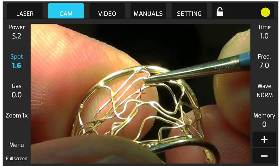
*Figure 15.1. When you press the Cam Tab you are able to view the weld area while still accessing weld parameter controls.*
