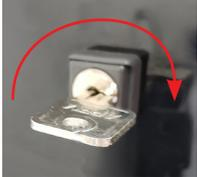
Figure 10.2. Turn the key clockwise to access the touchscreen controls.
