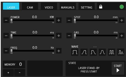
Figure 10.3. Touch the Start Button to adjust weld parameters and start welding.
