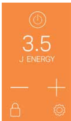
Figure 14.1 Set the Weld Energy Level to 3.5 J energy and then tap the Weld On/Off button so the power icon changes color from orange to gray.
