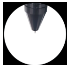
Figure 5.4. Only a small portion of the electrode should extrude from the holder.
