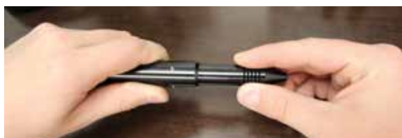
Figure 6.2. To install the electrode, first remove the Stylus Shaft (A) from the Stylus Hull (E) by pulling them apart.
