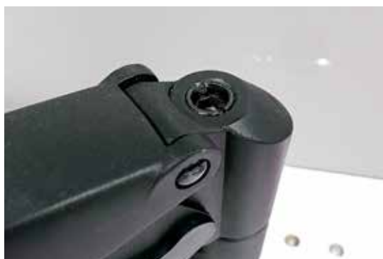
Figure 4.3. Adjust the tension of the Microscope Arm Assembly for more loose or more tight movement.
