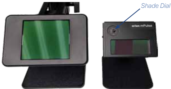
Figure 2.2. Upgraded Auto Darkening Lens (Left) and Regular Auto Darkening Lens (Right).
