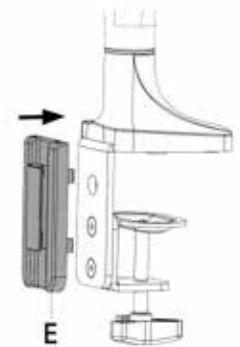
Figure 3.2. Cover the Clamp Mechanism (D) with the plastic cable guide cover (E).
