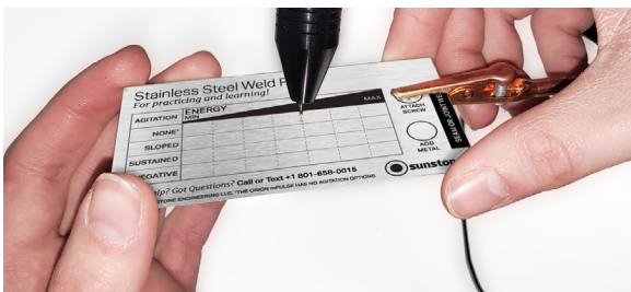
Figure 4.2 Attach the alligator clip to the welding plate. With proper eye protection, hold the welding plate with both hands and lightly touch the electrode to the welding plate. When the electrode contacts the welding plate, the welder will release energy and create a weld.
