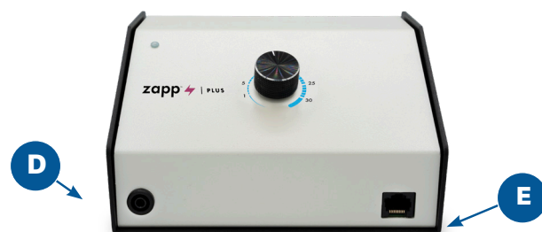
Figure 1.2. The back panel of the Zapp Plus. Grounding Port (D). Shutter Port (E).
