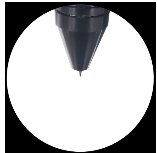
Figure 15.3. Only a small portion of the electrode should extrude from the holder.
