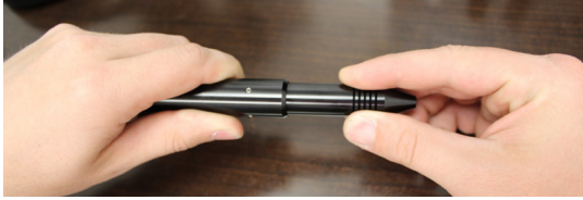
Figure 2.1. To install the electrode, first remove the Styling Shaft (A) from the Styling Hull (E) by pulling them apart.
