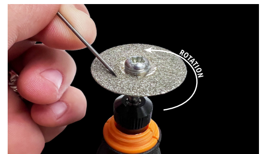
Figure 7.2. A sharp electrode tip improves arc initiation and results in a better overall weld.
