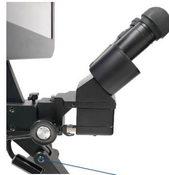
Figure 15.1. Turn this knob to adjust microscope focus. You'll find one knob on each side of the microscope arm.
