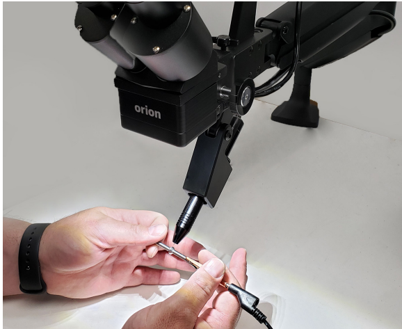
Figure 16.1. Rest your hands on the table and position the workpiece close to, but not touching the electrode. Then look through the microscope.
