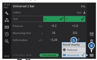
a) Press or (at the bottom right of the screen) to open the display selection window. The icon changes according to the selected display.
