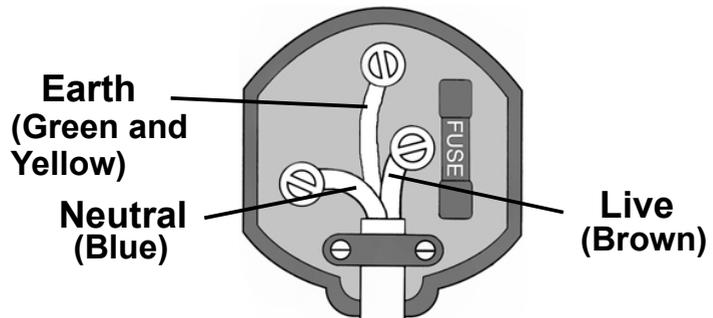
**make sure that the outer sheath of the cable is firmly held by the clamp**
