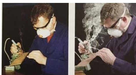
Soldering with and without Tyndall illumination – courtesy of the UK Health & Safety Executive (HSG258)
