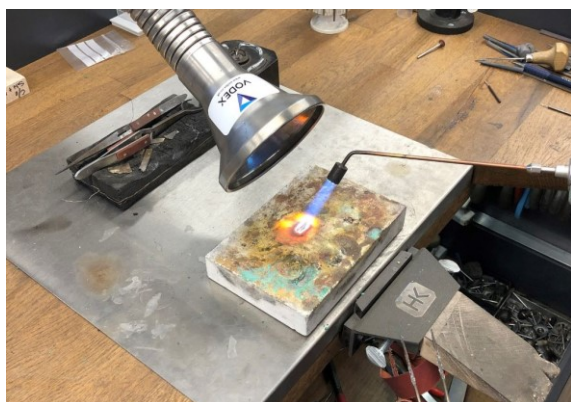
Flame/torch soldering with extraction
