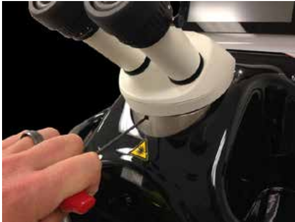
Figure 20.1. Before realigning the crosshairs, make sure the microscope is firmly attached to the welder.
