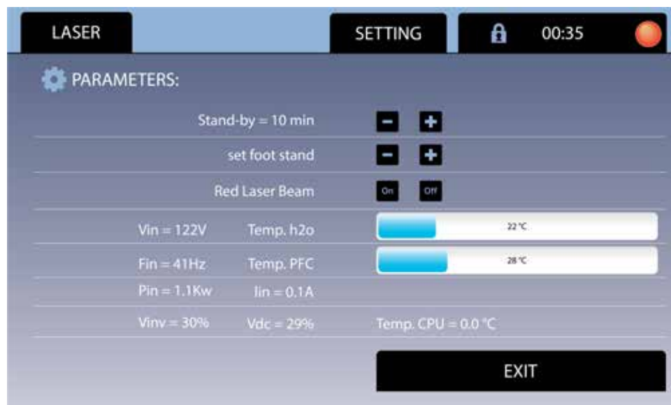
Figure 13.2. Press the Parameters Tab to set Stand-by Time, Platform Step, and view welder temperatures and other controls.
