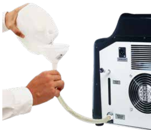
Figure 9.2. To fill the welder with coolant water, attach the funnel, tube, and connector to the bottom Female Connector "Remove Water" Port. Remove the Red Plug from the Upper Connector tube. Fill the welder with deionized water that comes with the Orion LZR laser welder.
