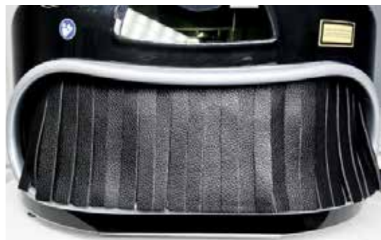
Figure 28.3. The leather strips at the front of the weld chamber prevent laser radiation from escaping the chamber while still allowing you to insert your hands and workpieces.
